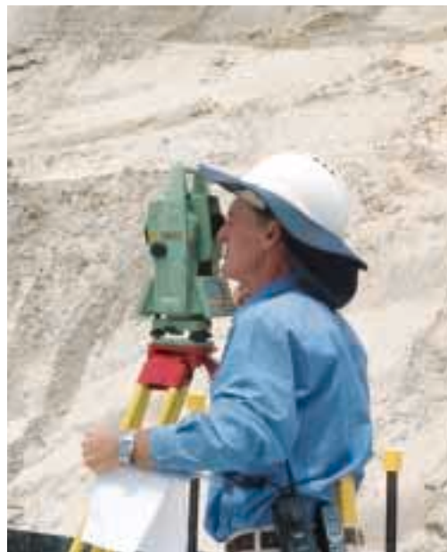
(above): Surveyor, Brian Rogers of Treasure & Associates uses a Leica TCR1101 for monitoring on the Q1 construction site.
