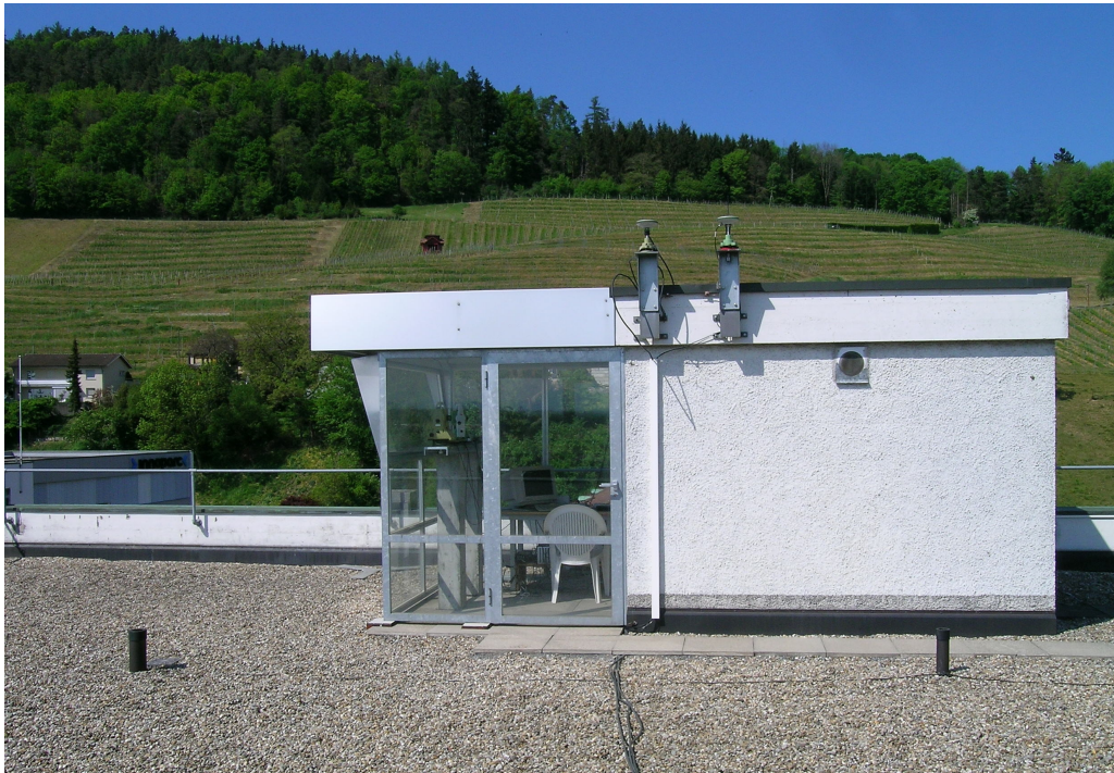
Figure 3 The measurement hut situated with the total station and the collocated GNSS antenna. The second total station and second GNSS antenna were not used in this experiment. One of the obstructing hills can be seen in the background.
