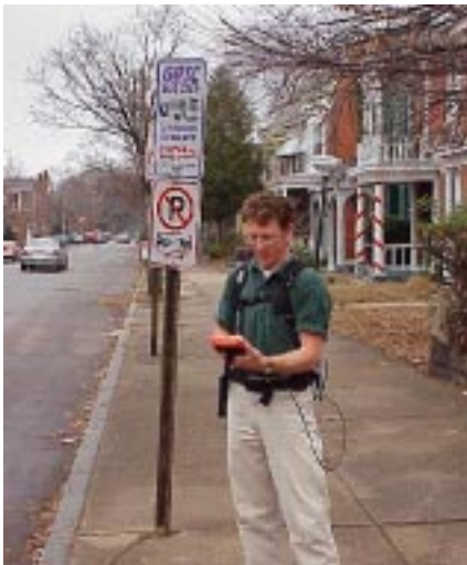
Jakob Helmboldt, GIS (Geographic Information Systems) Coordinator/Planner for the GRTC Transit System, uses a GS50 GPS/GIS receiver from Leica Geosystems to capture bus stop data in Richmond, Virginia.
