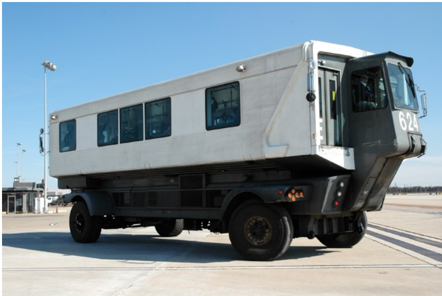
Top & bottom: Two styles of mobile lounges are currently used to transport passengers from the main terminal to outlying concourses.
