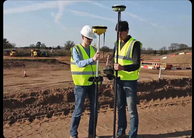
Foremen can use survey data in iCON site to stake out objects on site.
