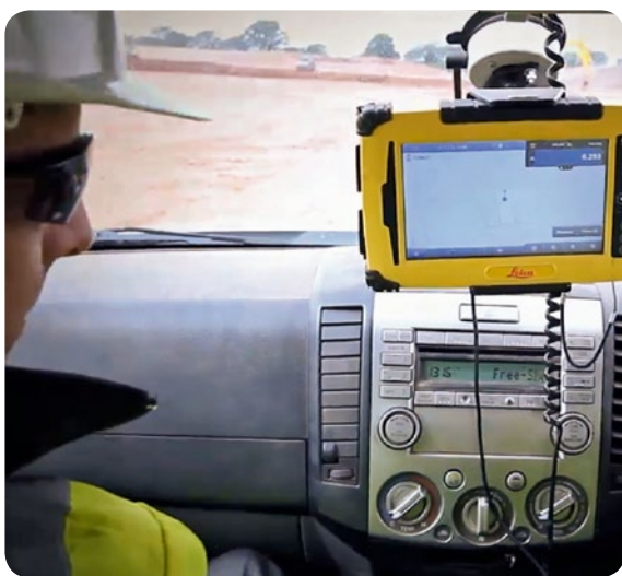
■ Height check: Leica iCON CC60 in the pick-up.
