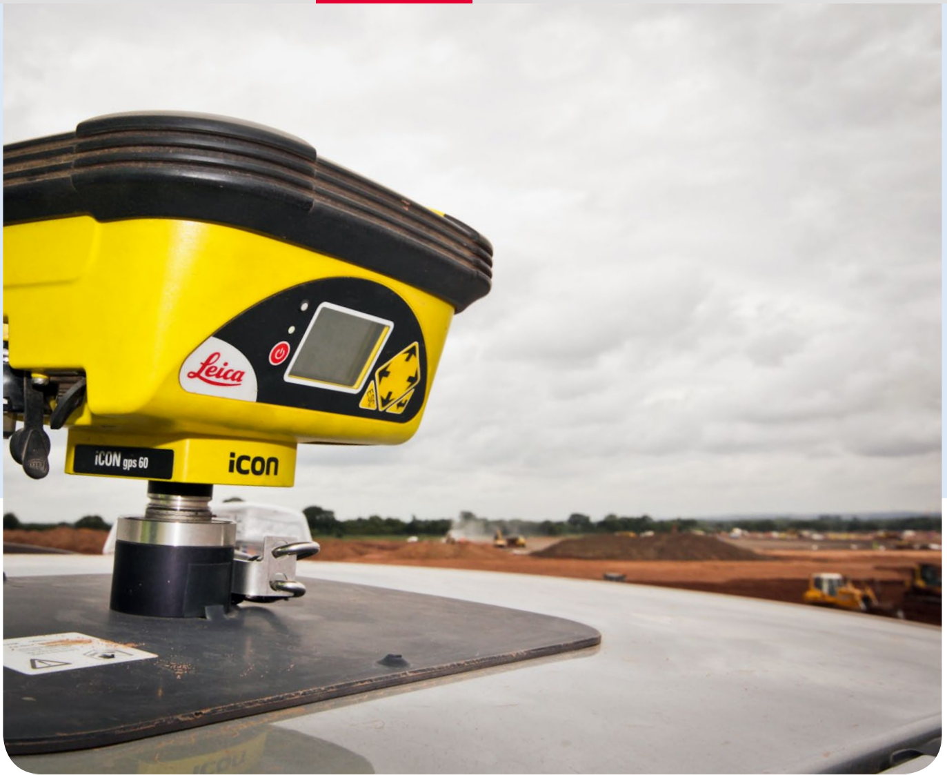
■ Leica iCON GPS 60 on the roof of the pick-up: the project manager can drive around the site, checking heights.
