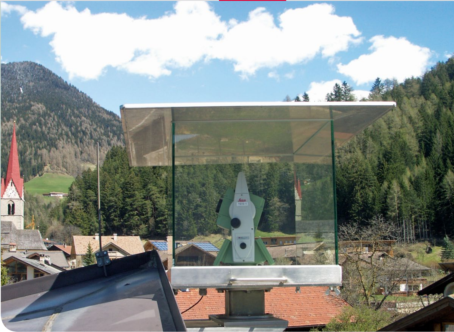
■ A Leica Viva TS15 Total Station monitoring surface movements in Mauils.
