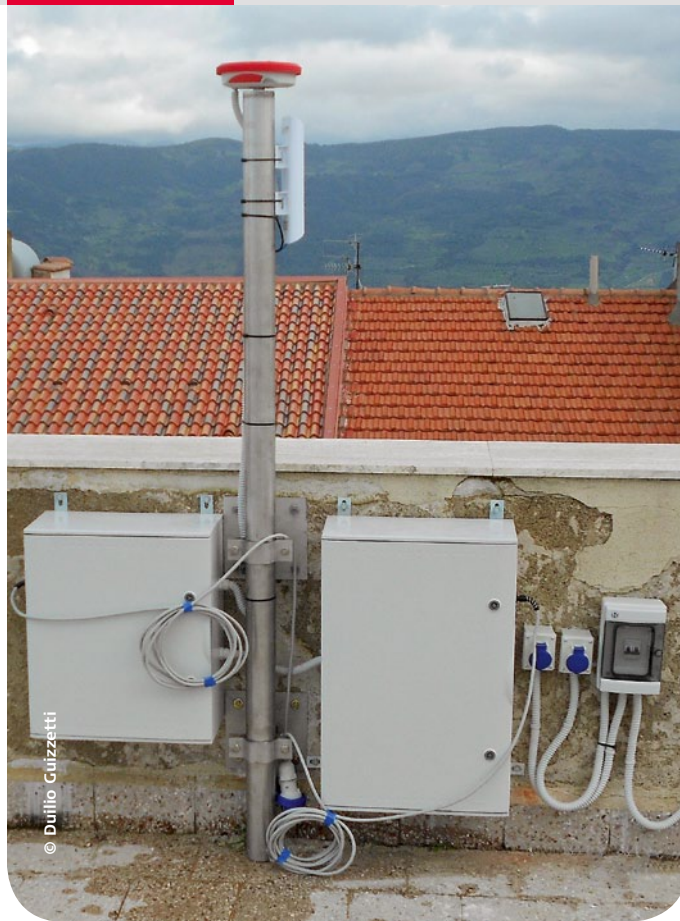
■ Station de surveillance GPS
